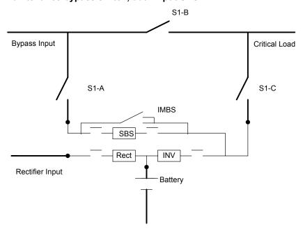
Figure 28 External maintenance bypass switch, single-input UPS
